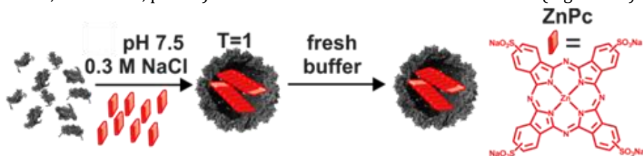
Figure 3.4. Schematic representation of the encapsulation approach of ZnPcs into CCMV by mixing ZnPcs and CP at pH 7.5.
